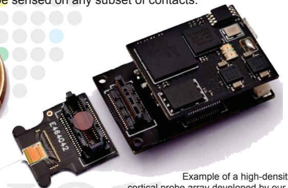
Example of a high-density intra-cortical probe array developed by our project partner imec. A similar system architecture providing an increased electrode count is addressed in NeuroSeeker.
